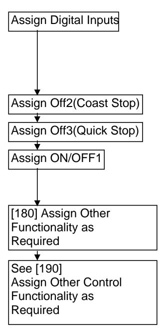
Digital Inputs/Outputs: Binector Assignments for Control may be made from Digital Inputs
